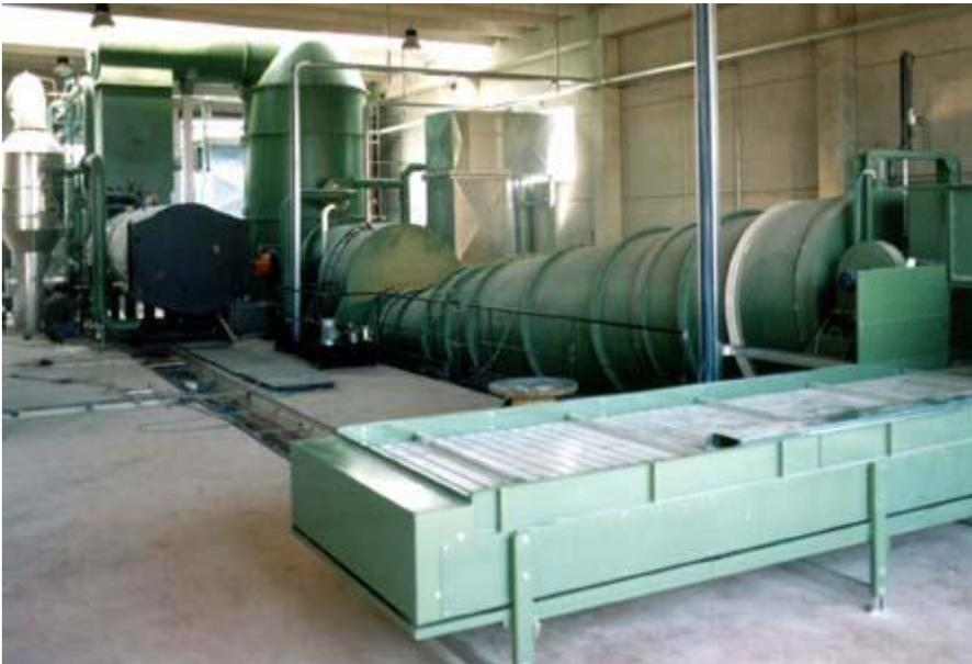
This series of plants has the highest destruction capacity available out of those made by Ciroldi S.p.A.: they feature constant running capacity and provide performance levels that generally range from 500 to 2000 kg/h, according to the type of waste. Thanks to their unique characteristics they can adapt to the
